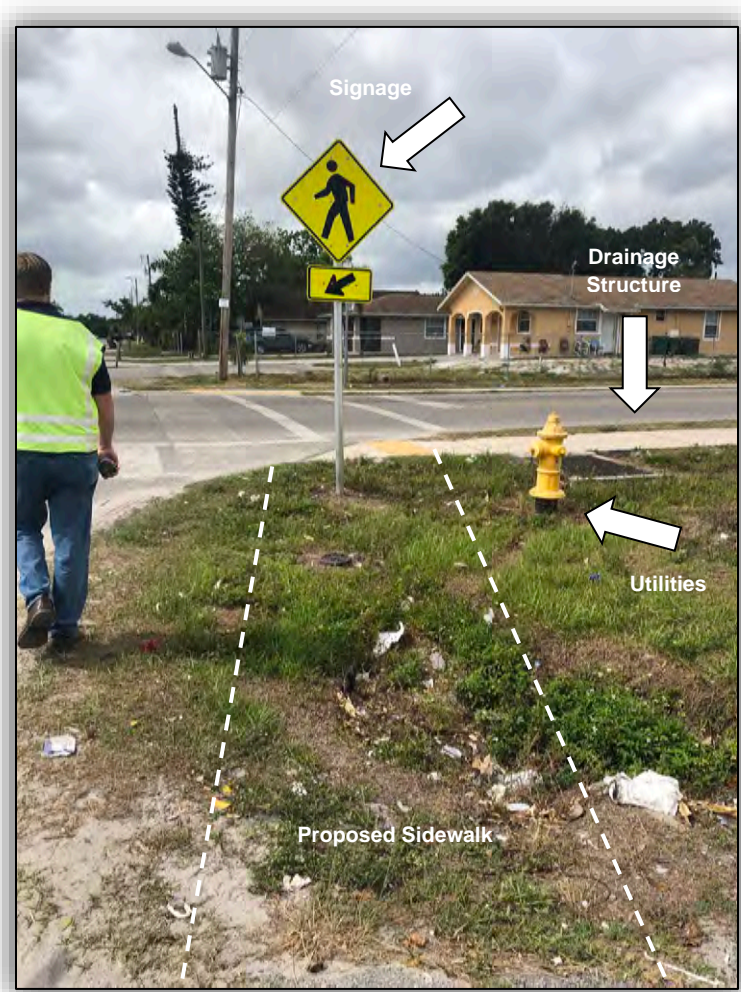
Figure 10-5: South 2 nd Street Sidewalk Connection
