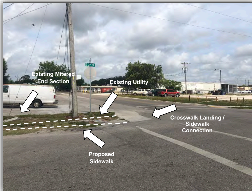
Figure 10-1: Sidewalk Connection / Crosswalk at Boston Avenue
