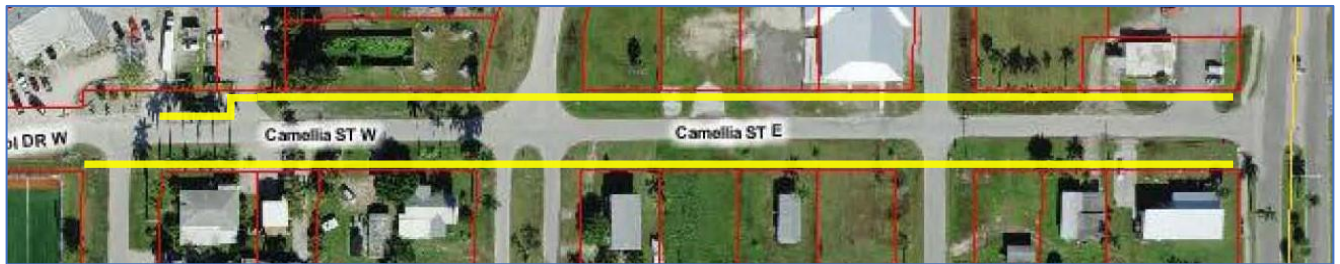
CAMELLIA STREET 75' ROW, 20' 2-LANE ROADWAY, SWALES ON SIDES
