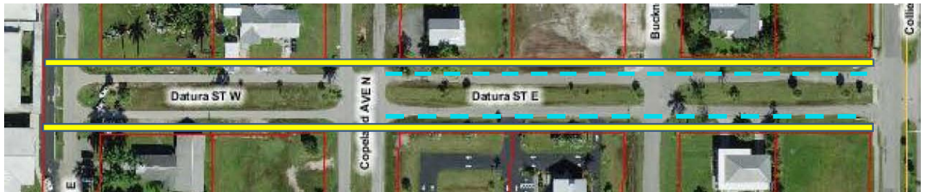
DATURA STREET – 100’ ROW, 2-LANE DIVIDED, SWALES ON SIDES
